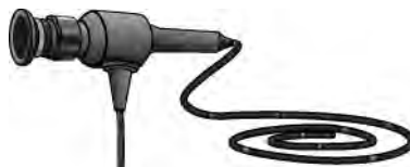
Figure 16.24 Endoscopes, such as the one drawn here, send light down a flexible fiber optic tube, which sends images back to a doctor in charge of performing a medical procedure.
