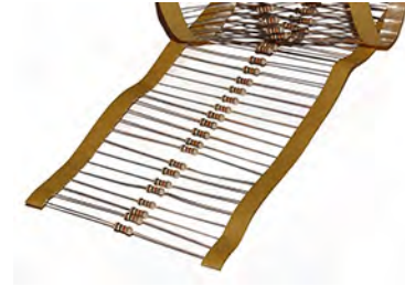
Figure 19.10 Some typical resistors. The color bands indicate the value of the resistance of each resistor.
