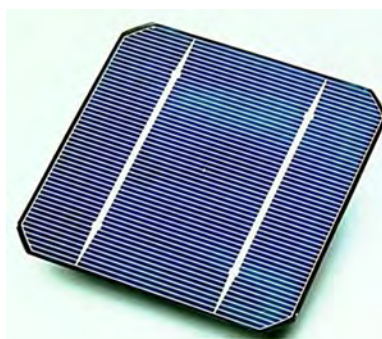
Figure 21.9 A solar cell is an example of a photovoltaic cell. As light strikes the cell, the cell absorbs the energy of the photons. If this energy exceeds the binding energy of the electrons, then electrons will be forced to move in the cell, thereby producing a current. This current may be used for a variety of purposes. (credit: U.S. Department of Energy)
