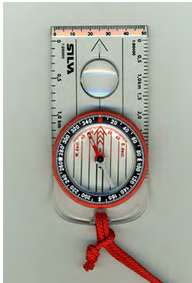
Figure 20.3 A compass is an elongated magnet mounted in a device that allows the magnet to rotate freely.
